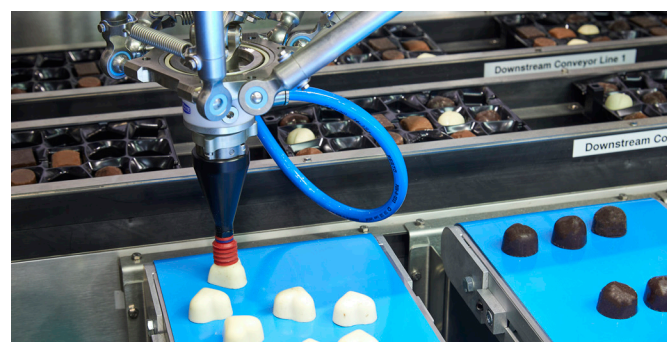
3-Axis Robotic Movement with Rotation
