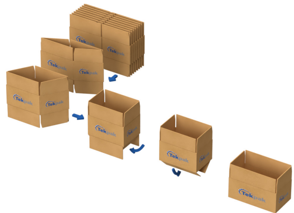
Case Erecting Sequence
