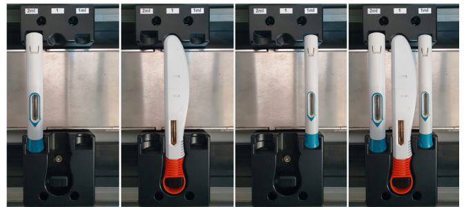
Custom Transfer Carriers for Handling Multiple Pen Formats
